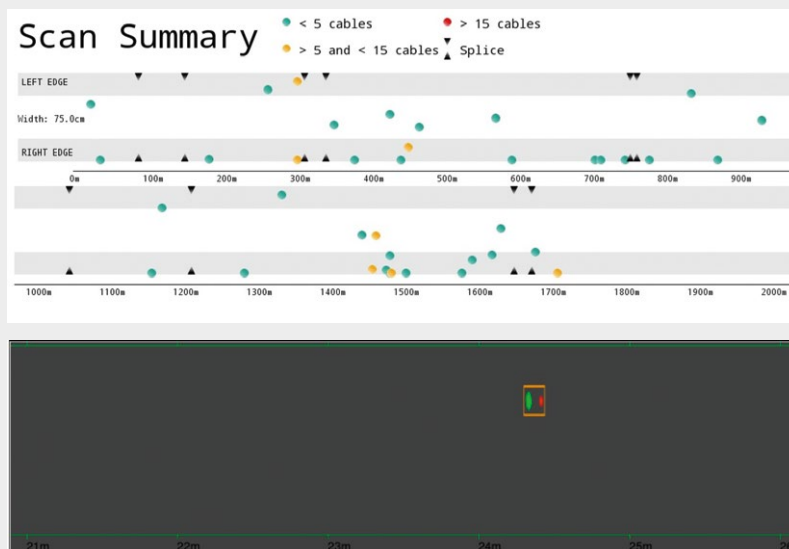
Image 1: Shows a steel cable broken on the left side of the conveyor belt at 24.4 meters from the starting point of the scan.
